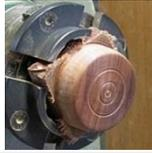
Some turners do the back of the pendant first. Put a few grooves to give it a nice finish look or even do off-center cuts. Do not sand this too fine, it could slide on the double-faced tape. Part off about a 1/4" disc.
