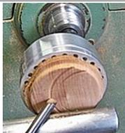
\* Slow the rpm's down so the lathe doesn't vibrate. If you have a variable speed, start with the very slowest speed and gradually turn it up. You can use a skew flat on the tool rest or a small detail gouge to make the cuts. Turn the lathe by hand and use pencil to mark desired cuts. You can erase pencil, you can't erase a cut! I like to do a cut 2 or 3 times to get a nice deep, clean cut.
