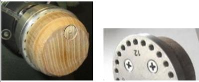
For a pendant, attach a solid waste block to the index faceplate using small wood screws. The size of the waste block should be slightly smaller than what you are turning. This makes it easier to grasp the finished piece to pull it off the waste block. The small circle is where I cut the hole for the cord on a pendant, with the mandrel in the #8 hole. This also helps line up the pendant if you need to finish the other side, too.
