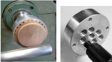
With the mandrel threaded into the middle hole on the off-center plate, clean up the surface of the pendant.
