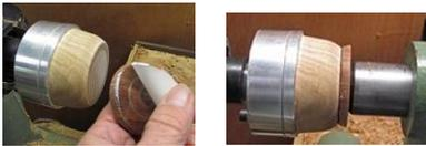
Attach 2 plates, make sure "0"s line up, use either sets of screws, it's a personal preference.
